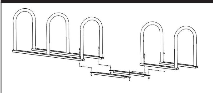
2.1: Slide each coupler into the C-channel so that holes on rack line up with slots in the coupler strap.
