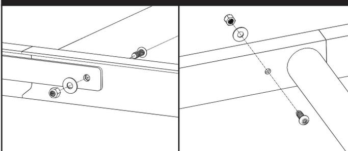
3.1: Put bolt through hole and slot from top of C-channel and put washer/nut combination on underside of C-channel. Hand tighten nut until bolt engages with plastic shield of nut. Repeat with all 4 bolts. Using 7/32" hex key to hold bolt, use 9/16" deep-well socket wrench to fully tighten.
