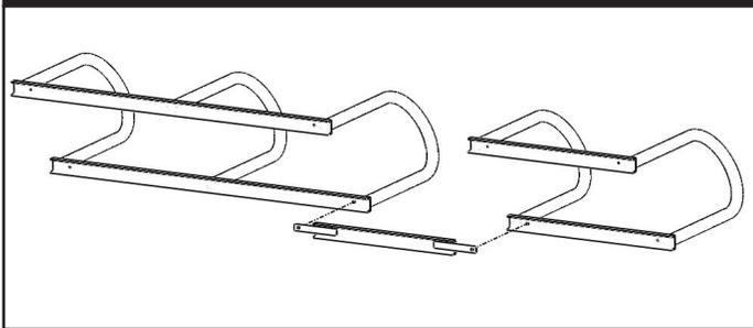
1.1: Place bike corral pieces in manner that you have access to top and underneath of C-channel. It is recommended that rack is placed on surface that prevents scratching of finish.
